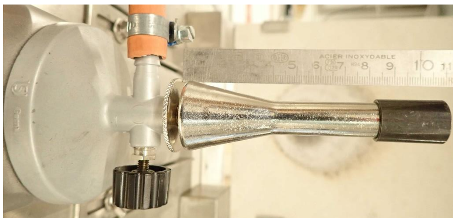
Figure 3: Teclu burner as used by nearly all of the participating laboratories. The actual total length of about 100 mm can be discerned.
