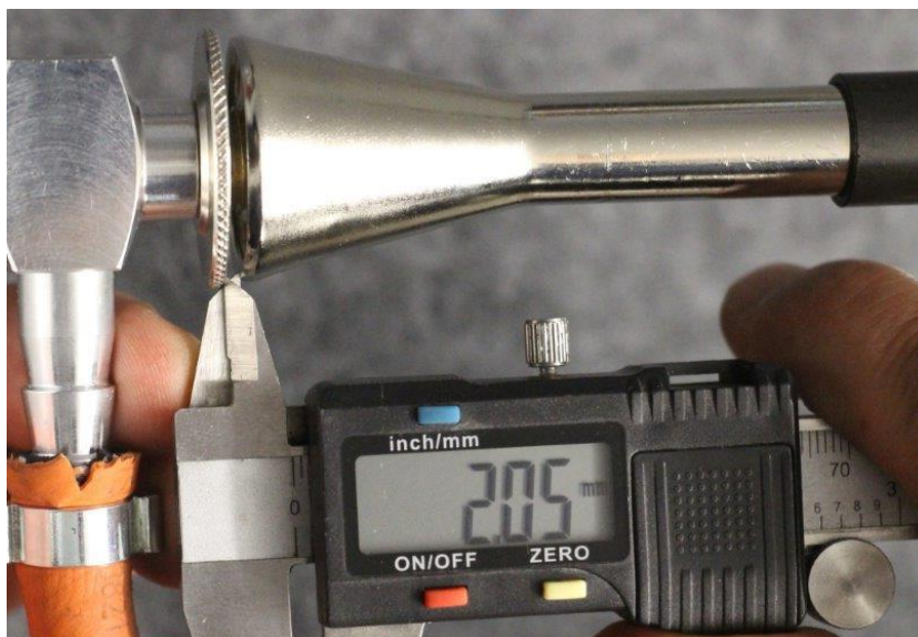
Figure 4: Air supply opening at the bottom of the burner.
